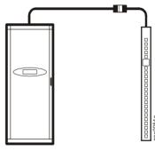
For dual-feed devices within a redundant system: attach a power cable from each PDU into two different Rack PDUs in the NetShelter VX Enclosure.
